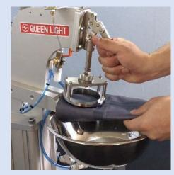
Free arm type - Good for testing a cylindrical part such as sleeve of rainwear.
